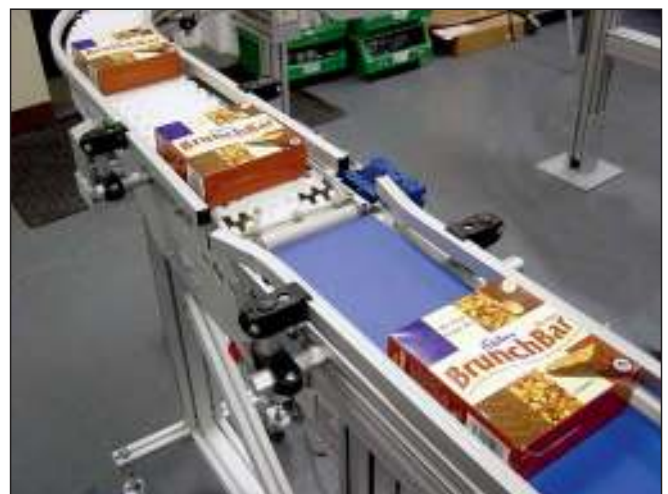
PACKING LINES. Chocolate bar packing line using a combination of Flex-Chain and belt conveyors. The line could be configured in five different layouts, allowing a number of different products to be run using one set of conveyors.
