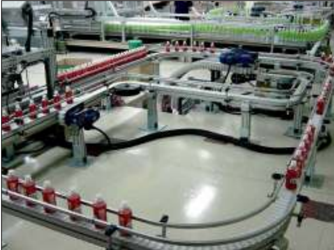
FLEX-CHAIN PLASTIC SLAT CONVEYORS. Ideal for efficiently conveying products between processes and machines. Very versatile, with large or small radius horizontal and vertical corners. Pinch grip system for vertical conveying. Also available in food quality stainless steel.
