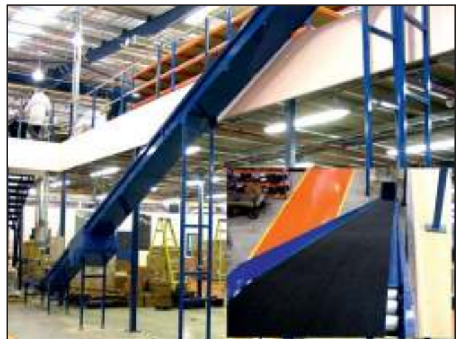
INTERFLOOR CONVEYORS. Very efficient method of transporting goods up to and down from a mezzanine floor. Uses a high grip belt and a powerful drive.
