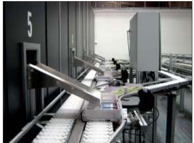
FLEX-CHAIN CONVEYOR SYSTEM. Transporting trays with an order of two spectacle lenses from five RAX Lens Stores to the dispatch department.
