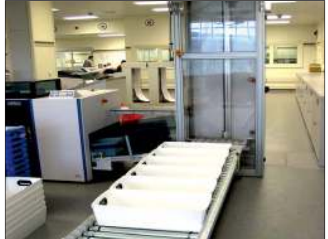
VERTICAL LIFTS. Available as a single vertical lift as shown above or as a continuous unit. Used for transferring to and from mezzanine floors or high level conveyors.
